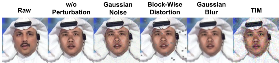
Figure 4: Samples of the perturbed images, including various corruptions at severity level 3 and adversarial example of TIM [10].
